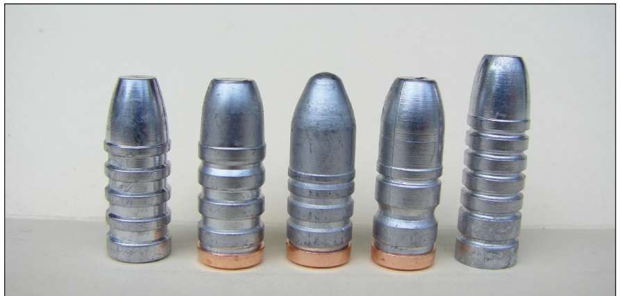
Cast bullets discussed include (from left): Lyman 319247, 157 grains; Accurate Molds 32-170B, 172 grains; Lee C324-175-1R, 173 grains; RCBS 32-170-FN, 178 grains; and Redding/SAECO 732, 200 grains.
